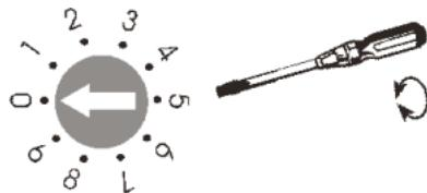
All transmitters and receivers within your system must be set to the same channel!
